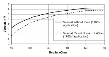
Fig. 3 V<sub>CEstat</sub> in dependence of R<sub>CE</sub>
