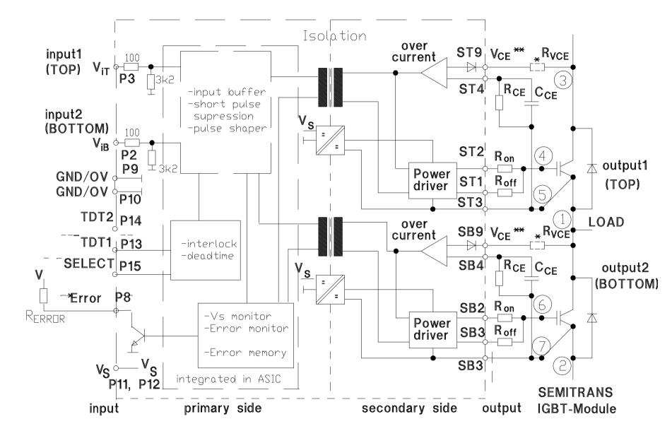
\* When SKHI 24 is driving 1700V IGBTs, a  $1k\Omega$  / 0,4W R<sub>VCE</sub>-resistor must be connected in series to the V<sub>CE</sub>-input.
