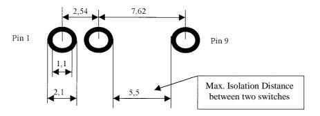
Fig. 7 Dimensions in [mm] for solder pads (as a proposal for a design) and solder pad gaps (partial drawing) with maximum distance between two switches
